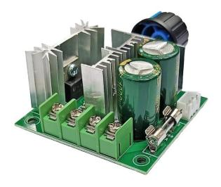
The DC Motor Speed Controller allows controlling direction of a DC motor using a Pulse-Width-Modulated (PWM) DC voltage with a Duty Cycle fully adjustable from 10%-100%. The motor speed controller can provide a continuous current of 8A to your DC motor or other DC load. The circuit also includes a 10A fuse, with the reverse connection of power supply and control voltage over-voltage protection function.
